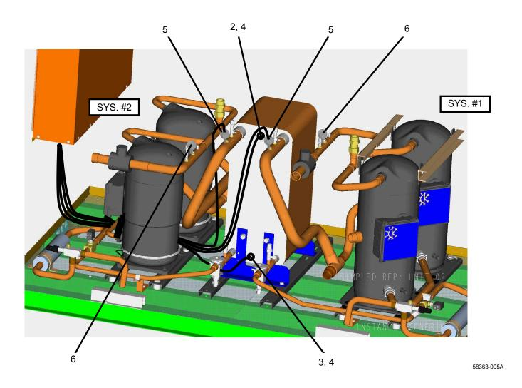
FIGURE 18 - TEMPERATURE SENSORS AND TRANSDUCERS
