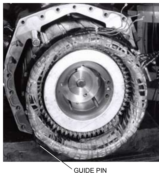
FIG. 44B – REMOVING THE STATOR (Horizontally)
