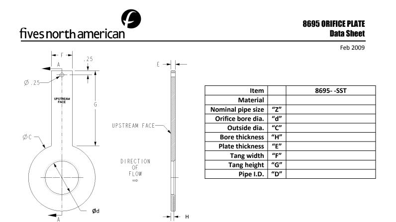
Tap Type must be specified. Note that flange taps and D,D/2 Pipe taps must be selected with consideration for the physical restraints of certain pipe sizes and flange thicknesses. For example a D/2 pipe tap would not fit in a 1" pipe due to flange thickness. Corner tap flanges (not shown) are available upon special request for  $\frac{1}{2}$ ",  $\frac{3}{4}$ " and 1" sizes.
