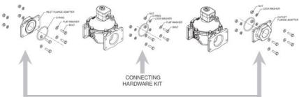
INLET / OUTLET FLANGE ADAPTERS AND HARDWARE
