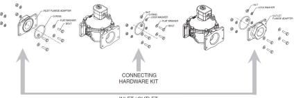
INLET / OUTLET FLANGE ADAPTERS AND HARDWARE
