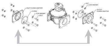
INLET / OUTLET FLANGE ADAPTERS AND HARDWARE KIT
