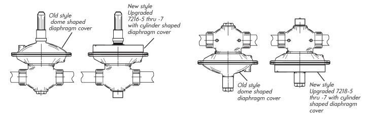
For sizes -5, -6, -7, old style regulators require an upgrade kit (-UK) which includes the cylinder shaped diaphragm cover.
