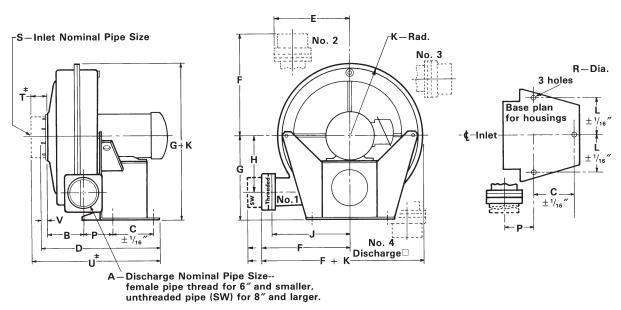
All dimensions are in inches. Dimensions shown apply only to blowers with T-frame motors. Consult North American for dimensions of blowers with other motors.
