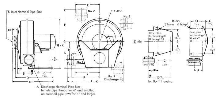
All dimensions are in inches. Dimensions shown apply only to blowers with T-frame motors. Consult North American for dimensions of blowers with other motors.
