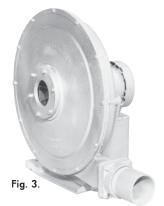
"SW" means sleeve or weld. A flexible rubberized sleeve (Bulletin 2947) can be slipped over an SW connection and clamped to prevent leaks. A flexible connection does not transmit vibrations or stresses as do welded or threaded connections. Blowers are not designed for imposed loads from hard pipe connections and should not be "hard" piped except under unusual circumstances.
