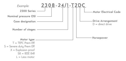
**Motor Electrical Code:** if this position is blank, this indicates standard voltage which for 60 Hz would be 230/460 volts 60 Hz 3 phase volts. Other typical electrical codes include:
