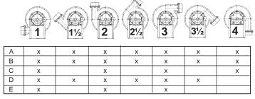
The letter assigned to each blower below indentifies the standard discharge positions available. Contact the Product Manager for other discharge positions (at extra cost and longer delivery).
