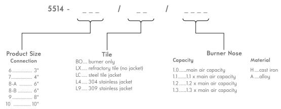
Example 1 5514-8-A/LC/1.2A Fireall oil burner complete with carbon steel jacketed tile and 1.2 capacity alloy nose
