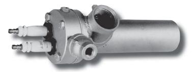
115/230/1/60. This oil pump is equipped with ½" NPT ports and an internal pressure relief valve. We recommend the use of a system oil pressure regulator (7142-01-70) and a system relief valve (7177-01-150) with a return oil line to the oil reservoir.
