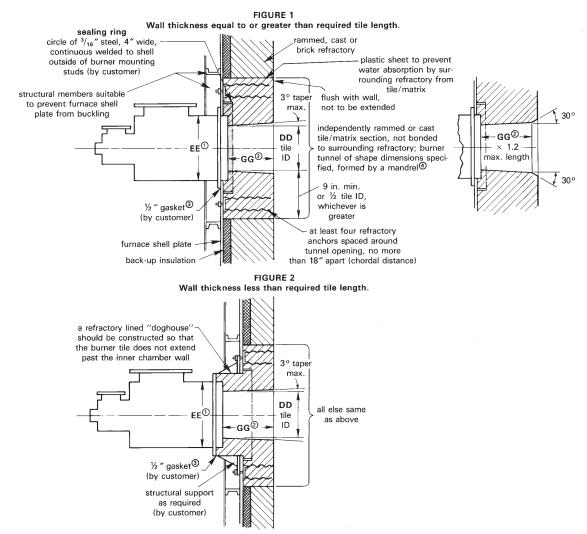
D Furnace opening should be ½" larger than dimension EE for -8 thru -14; ¾" larger than dimension EE for -16 thru -24.
