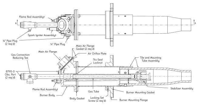
† When replacing igniter and/or flame rod assemblies in the field, it is recommended that the burner body be removed from the tile mounting tube flange to ensure insertion into the access holes provided and not into one of the air tubes on either side.
