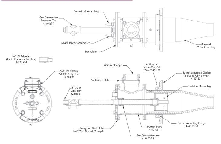
+ When replacing igniter and/or flame rod assemblies in the field, it is recommended that the burner body be removed from the tile mounting tube flange to ensure insertion into the access holes provided and not into one of the air tubes on either side.
