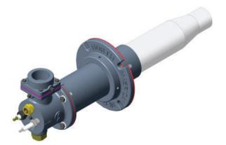
Enhanced temperature uniformity and heat transfer promoted by recirculation of combustion products, improve both product quality and productivity in many kilns and furnaces. True high velocity burners entrain and recirculate products of combustion (poc) volumes seven or more times greater than the actual tile exit gas volume, potentially eliminating the need for excess air operation or hot gas recirculation fans.
