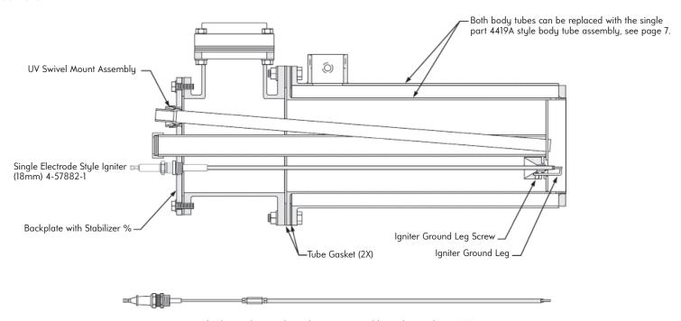
Obsolete multi part electrode Igniter Assembly, replace with 4-57882-1
