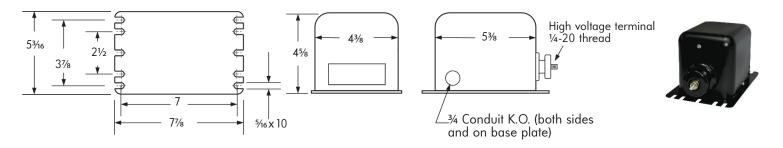
Use 1/4" ring tongue connector for 4085 connector (type "B")
